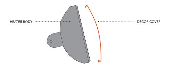
1. START BY INSERTING THE DÉCOR COVER TO THE BOTTOM OF THE HEATER'S INDENTED SLOT.
